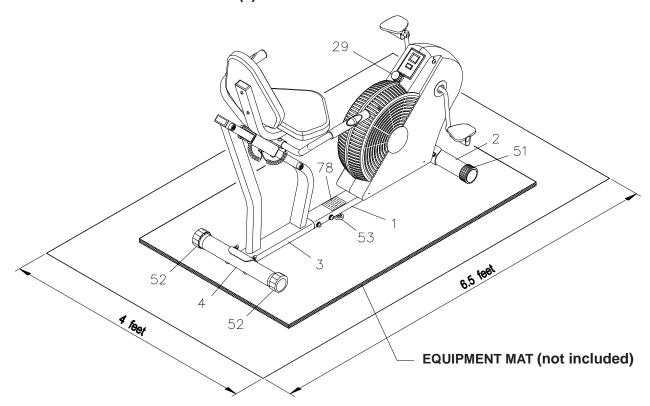
To level the Air Fusion 4525 Bike, first screw the STAND(53) located in the middle of the FRONT FRAME(1) all the way up into the FRONT FRAME(1) so that it is not touching the floor. Adjust the two LEVELING CAPS(52) on the REAR STABILIZER(4). When the LEVELING CAPS(52) are adjusted and the Air Fusion 4525 Bike is stable, rotate the STAND(53) to make it contact with the floor.
